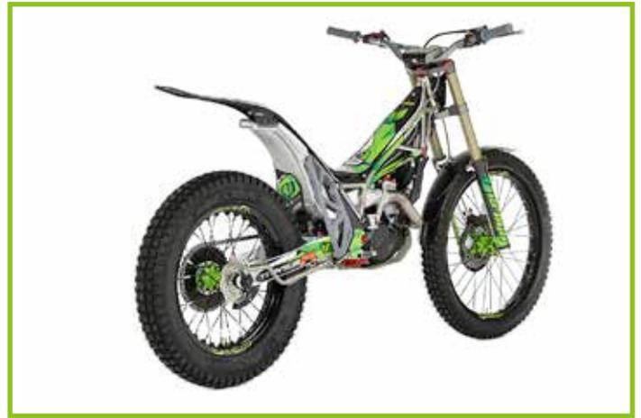
Within its new features we can find the Titanium GR5 tubular frame that weights only 2.100kg. In addition, all the screws and foot pegs supports are also on titanium, which lows 500gr its heaviness. The magnesium swing arm contributes as well on keeping this Titanium R's 2018 weight heft, adding only 1,600kg.
